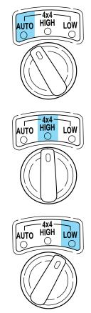
The vehicle should not be operated in 4WD HIGH and 4WD LOW on dry or merely wet pavement. Doing so will produce excessive noise, increase tire wear and may damage driveline components. These modes are intended for use only on consistently slippery or loose surfaces.
